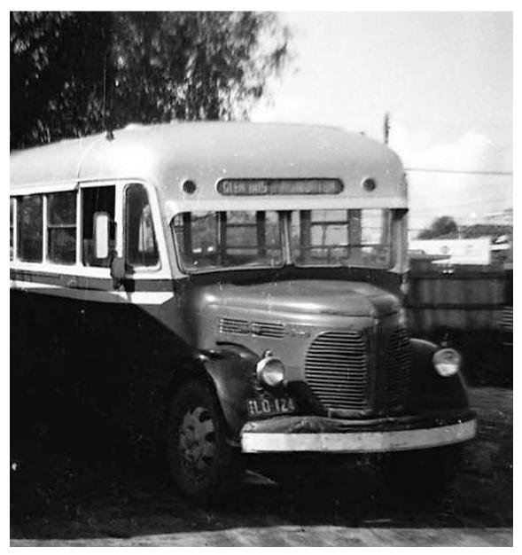
ME-673 1948 Reo / Ansair Body / Perkins diesel engine (originally Reo petrol).
